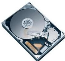
What we have now are smaller cousins to those huge main-frame disks. They are constructed of thin aluminum or glass disks (platters), 3 1/2" diameter, which are coated with a very thin layer of magnetic material. Similar to a record player's tone arm, a read/write (R/W) head at the end of an arm
